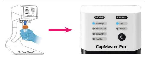
Press the button for 3 seconds to select the different cycle time. The LEDs will blink when setting the cycle time.
